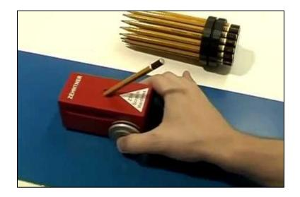
Interpretir This simple metal "car" produces more consistent test results by providing The point consistency in the angle and pressure during the Pencil Hardness test procedure ratch the surface is the reported surface harness level.
