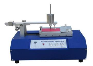
This device uses varying pressure, and measures the force required to scratch the surface.
